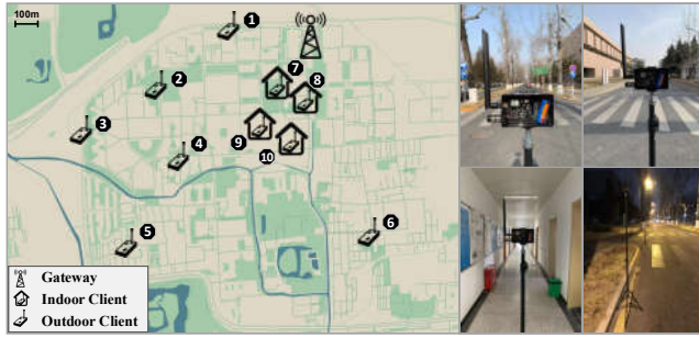
Figure 20: Campus-scale LoRa testbed deployment.
