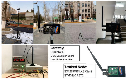
Figure 11: USRP N210 based gateway and COTS LoRa nodes deployed in a campus environment.
