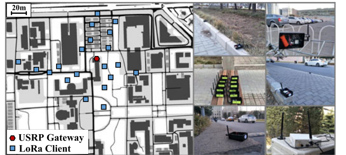
Fig. 13. The outdoor deployed LoRa network, each sensor node transmits temperature and humidity data by LoRa packets periodically.
